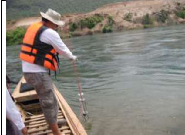
1. Sampling of water from different depth at sampling station
