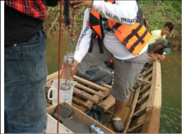
2. Gathering of sampled water from each grab into plastic jar
