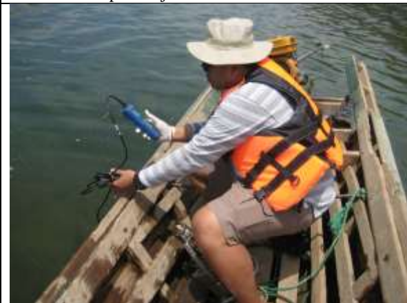
4. In situ measurement of water quality at sampling station
