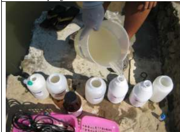
3. Pouring of sampled water to containers and fixation prior store in cool container
